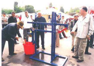
Picture 3. Water pump with pendulum, Novi Sad, 2003 Free Energy conference in Rome 2010 - Pump with Pendulum on the first page - http://www.veljkomilkovic.com/rucnaPumpaEng.html
